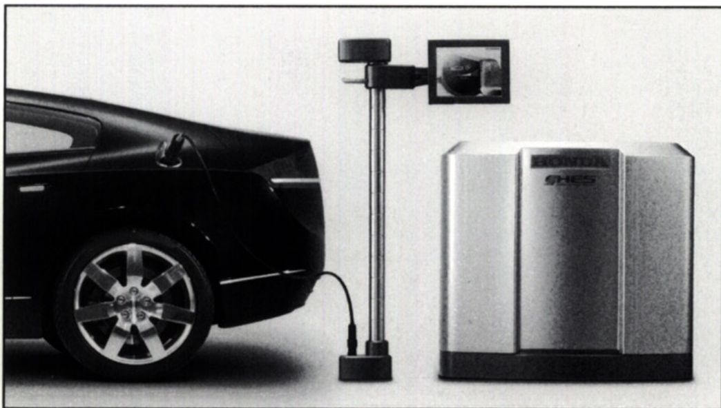
Honda Hydrogen Fuel Car, FCX, with home refueling unit, being rushed into development. ( Courtesy of the American Honda Co. )
