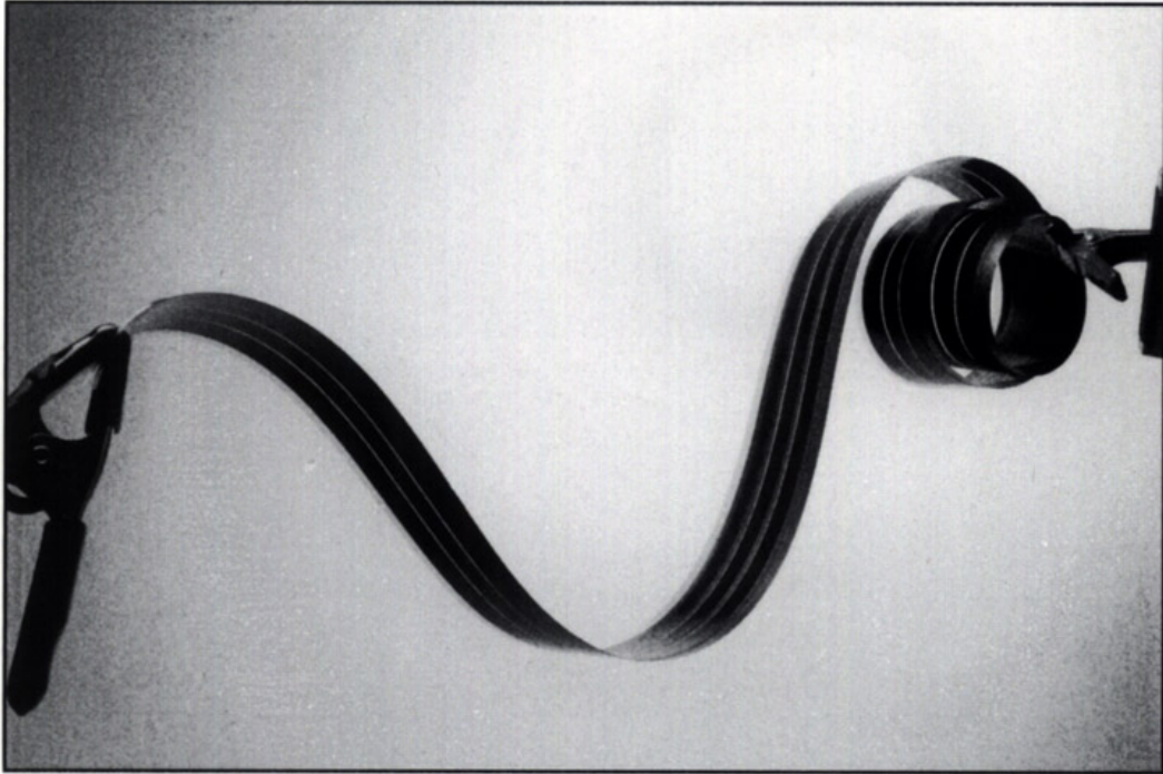
This is a strand of film with embedded Konarka nanosolar. ( Courtesy of Konarka Technologies, Inc. )
